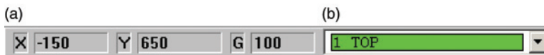
Figure 3-13 Cursor location and grid indicators and layer controls. (a) Cursor coordinates and placement grid. (b) Active layer dropdown list.
