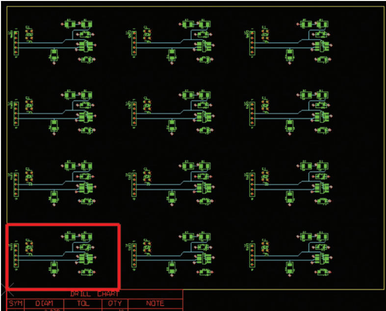
Figure 11-38 The panelized board design.
